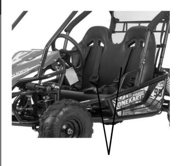
Never start the go kart without the operator and passenger wearing the seat belt harness in the appropriate manner.
