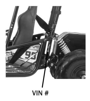
The Vehicle identification number is needed when calling for parts, service center help or when registering your Go Kart. Locate the number and list the number below for your reference.
