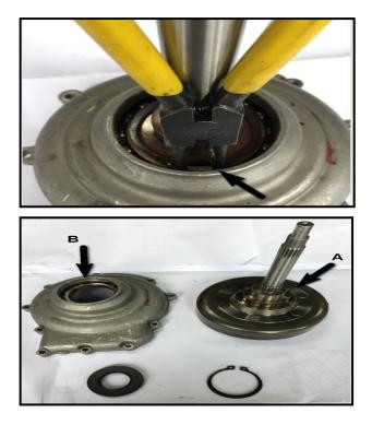
Remove the snap ring as shown from the groove in the clutch housing and remove the clutch housing (A). Separate the clutch housing (A) from the bearing housing (B).
