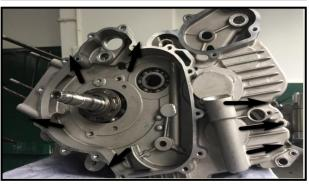
• Remove the gear position switch mounting bolts (A), Switch (B) and O-ring.
